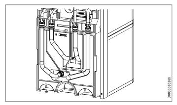
► Release the sensor lead from the guide groove.
