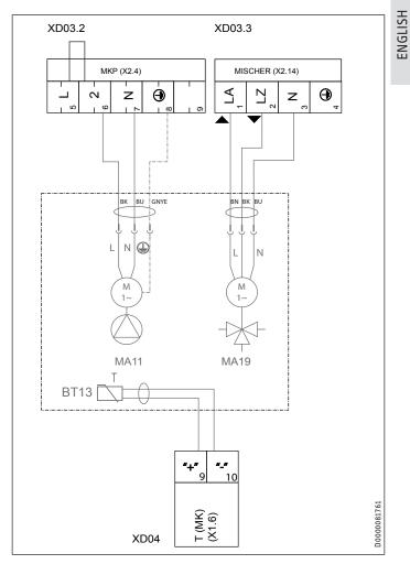
► Wire up the heating circuit pump and 3-way mixer (see chapter "Installation / Electrical connection / Control voltage").
