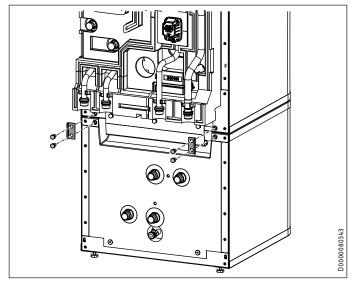
▶ Release the 4 screws on the tabs at the front of the appliance.
