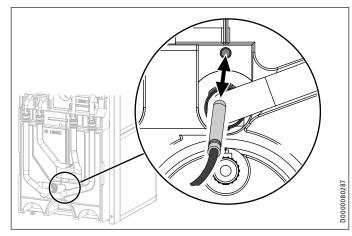
▶ Pull the "heating sensor" out of the buffer cylinder.
