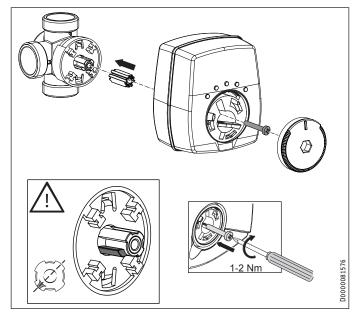
► Check the position of the 3-way mixer shaft. Adjust the position if necessary.
