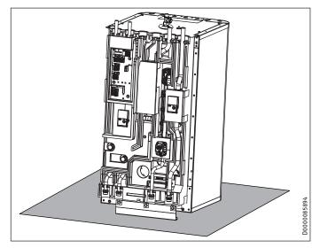
► Place the upper section of the appliance on a base to prevent damage.
